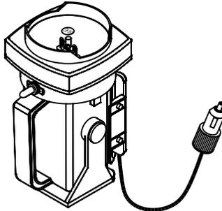
Mount the charger-base in a vehicle in an upright position (as in illustration) near the cigarette lighter or other accessory outlet and plug the DC charger into the receptacle.
