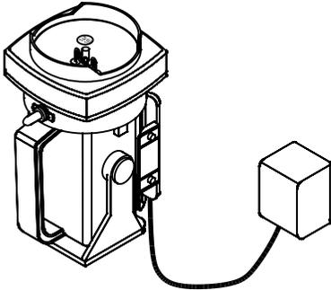
Mount the charger-base in an upright position (as in illustration) near a 110-volt receptacle. Plug the AC charger into the receptacle. Red light indicates the battery is charging.
