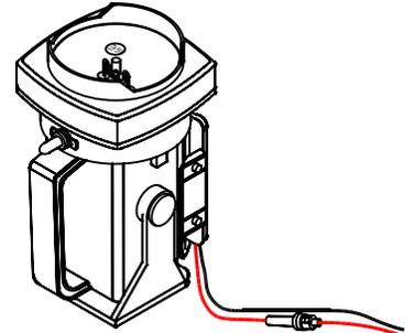
Mount the charger-base in a vehicle in an upright position (as in illustration). Connect the Black wire to ground and the Red wire to a constant +12-volt positive.
