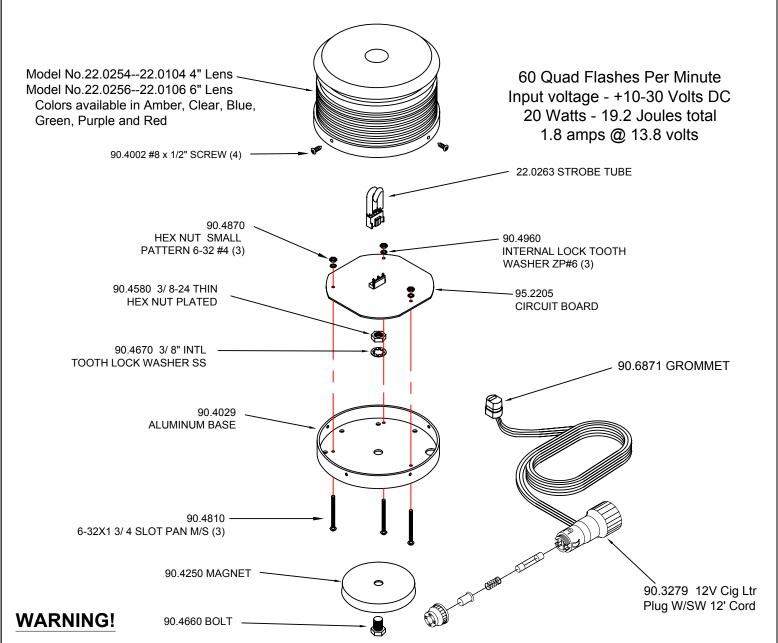
Do not install this product or route any wires in the deployment area of your air bag. Equipment mounted or located in the air bag deployment area will damage or reduce the effectiveness of the air bag, or become a projectile that could cause serious personal injury or death.
