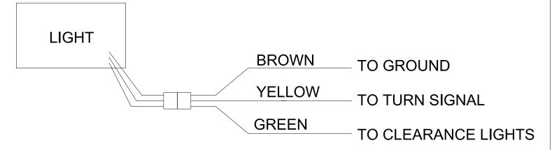
**Caution:** Do not mount where light beam is directed into passing lane of traffic or to the rear of the trailer.
